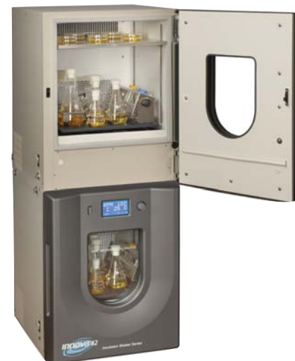
Shown stacked two units high. Stationary shelf and internal power receptacle are standard.
