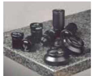
Additional eyepieces or lenses allow for the degree of magnification to be increased or decreased.
